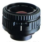
Focal length 105.5mm Minimum f/stop f/32 Lens construction 4-6 Standard 5X magnification Usable 2X ~ 10X magnification range Covering power 51° Correction 380 ~ 700mu wavelength range 2.4 in. x 3.5 in. Format size (60 x 90mm) Max. negative 4.7 in. diagonal (120mmø) 3.9 oz. (110g) Weight 1.6 in. Length (a) (40mm)
