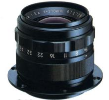
Focal length 210mm Minimum f/stop f/45 Lens construction 4-6 Standard 4X magnification Usable 2X ~ 8X magnification range 54° Covering power Correction 380 ~ 700mu wavelength range 5 in. x 7 in. (130 x 210mm) Format size Max. negative 10.6 in. diagonal (270mmø) 21.2 oz. Weight (600g) 3.0 in. Length (a) (77mm) 3.2 in. Diameter (b) (82mm)
