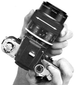
of the lens. As the image is constantly viewed at the maximum aperture setting (i.e., f/4), the depth of field is minimized so that the image snaps in and out of focus rapidly and distinctly.
