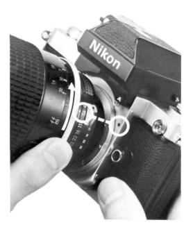
Position the lens in the camera's bayonet mount, aligning the mounting indexes on the camera and the lens. Twist the lens counterclockwise until it clicks into place.
